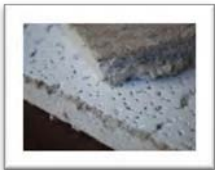
Perlite used in ceiling tiles dampens noise.
